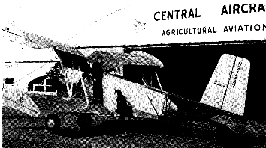
The Air Tractor is the type of aircraft that operators seem to believe may eventually develop for the future. An example of a utilitarian design with frills cut to a minimum. This plane is basically an airborne farm implement, capable of carrying large payloads of either dust or spray
